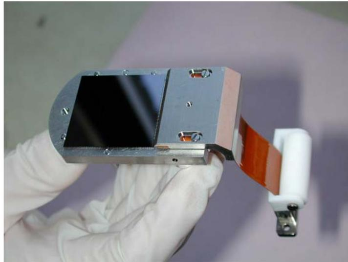
**Figure 15** The SECCHI EUVI CCD in its carrier, with the flexible printed circuit harness attached. The overall size of the CCD chip is about 28.1 x 30.3 mm. The CCDs used in the HI instruments differ only in the presence of an AR coating.
